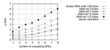
Fig. 4. Measurement of Competing Writes to a Cache Line
